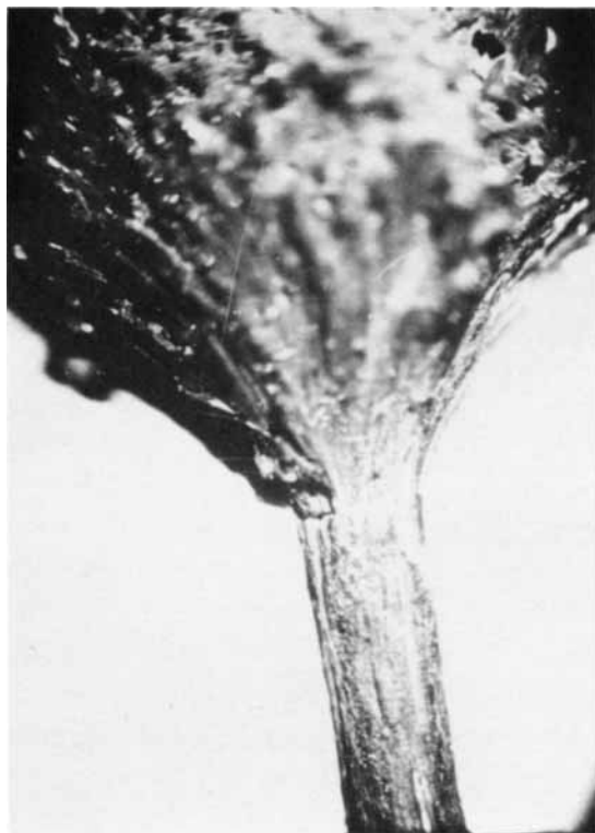
Figure 4 The appearance of sample obtained with using a sectional capillary (entrance angle 180^\circ ) after washing out PSPh and removing a PES from stagnant zones. Magnification 15\times .
